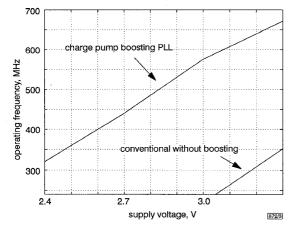
Fig. 3 Maximum PLL lock frequency against supply voltage
